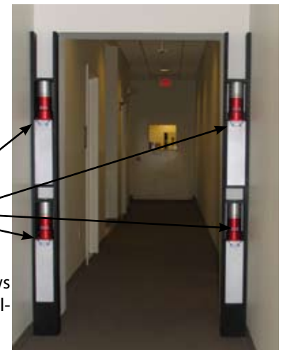
The photo above shows a high sensitivity detector, a 10 \times 10 \times 40 \text{ cm}^3 ( 4 \times 4 \times 16 ) NaI(Tl) "bar."
