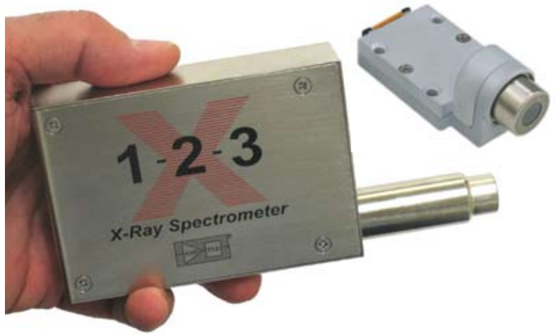
Figure 2. X-123 X-Ray Spectrometer and OEM configurations.
